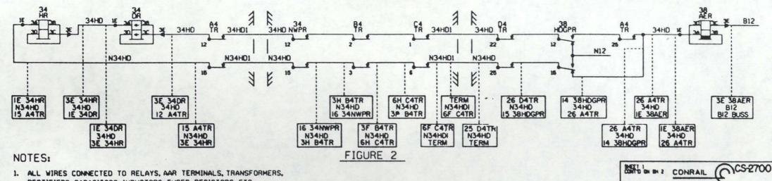
ALL WIRES CONNECTED TO RELAYS, AAR TERMINALS, TRANSFORMERS, RECTIFIERS, CAPACITORS, INDUCTORS, FUSES, RESISTORS, ETC., SHALL BE TAGGED AS SHOWN IN FIGURES 1 AND 2.
