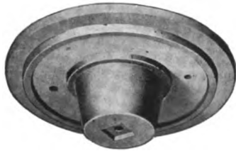
Porcelain Cover with Integral Lug extending below Solution Line to prevent internal Short Circuiting at Solution Level.
