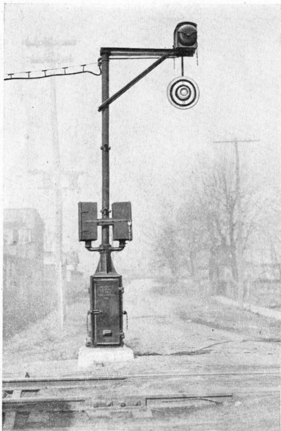
Installation of Magnetic Flagman (two position, lower quadrant), on Louisville & Nashville R. R., Lebanon, Ky.
