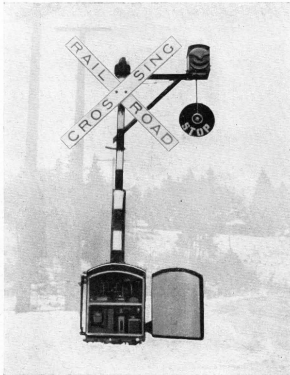
Installation of 8-volt D.C. Magnetic Flagman (two position, lower quadrant), on Northern Pacific R. R.
