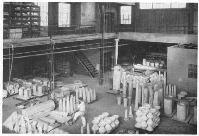
A CORNER OF THE NEW CASTING DEPARTMENT. IN THE BACKGROUND THE CORE IS BEING DRAWN FROM AN OIL-FILLED BUSHING PORCELAIN
