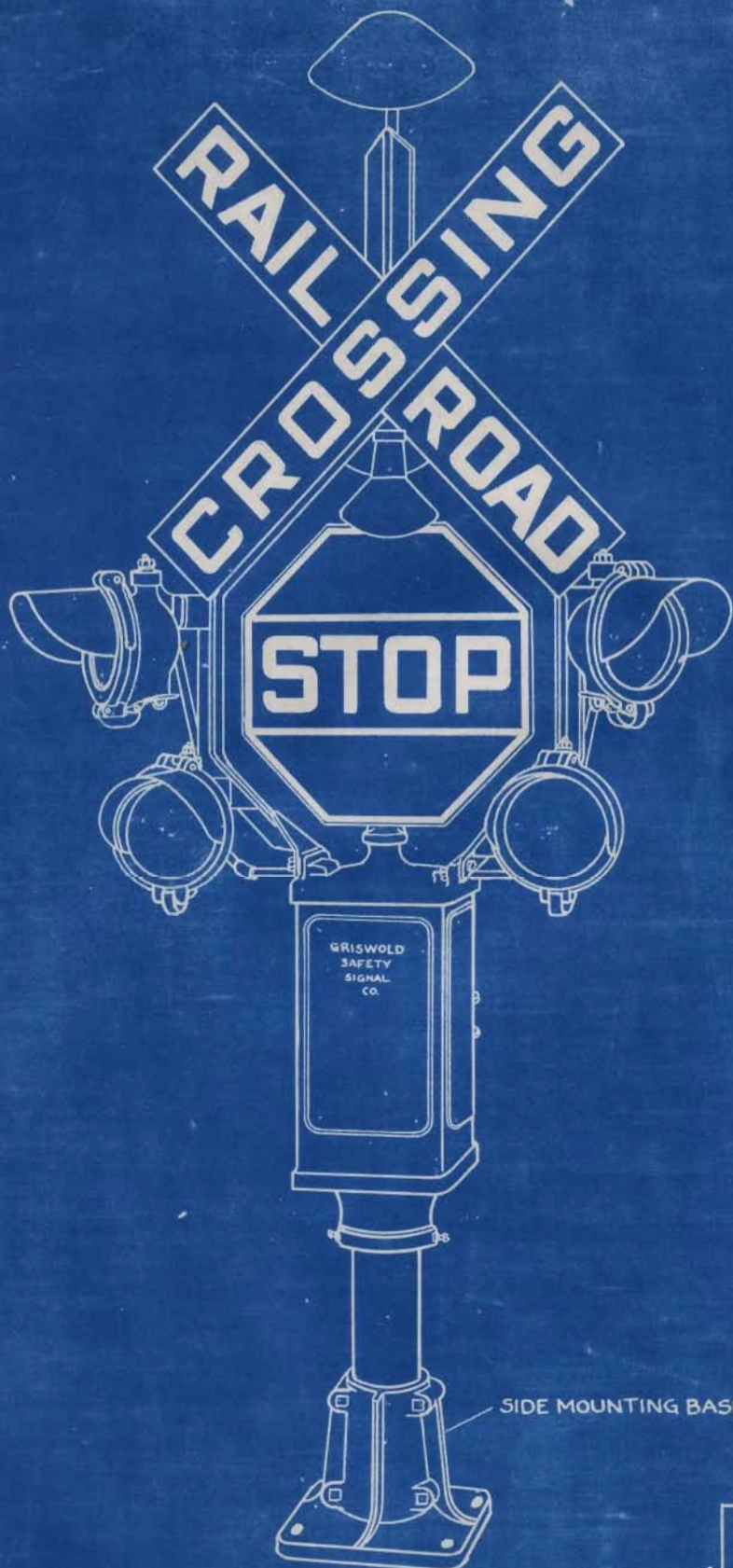
HIGHWAY CROSSING SIGNAL WITH FOUR ADJUSTABLE FLASHING LIGHTS FOR PROTECTING A CROSSING WITH ROADS APPROACHING AS SHOWN IN THE KEY MAP AT THE RIGHT. SPECIFY CENTER OR SIDE MOUNTING BASE
