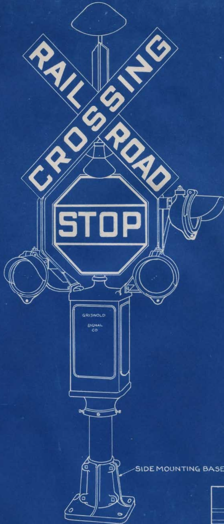
HIGHWAY CROSSING SIGNAL WITH THREE ADJUSTABLE FLASHING LIGHTS FOR PROTECTING A CROSSING WITH ROADS APPROACHING AS SHOWN IN THE KEY MAP AT THE RIGHT SPECIFY CENTER OR SIDE MOUNTING BASE
