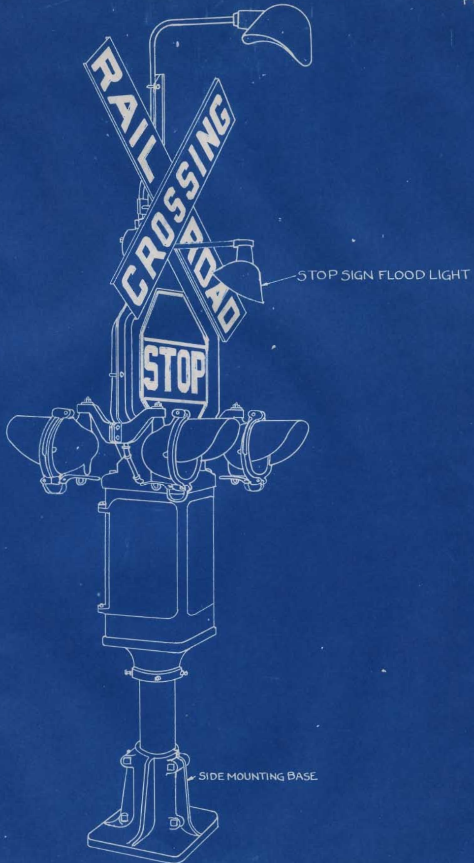
HIGHWAY CROSSING SIGNAL WITH STOP SIGN FLOODLIGHT
