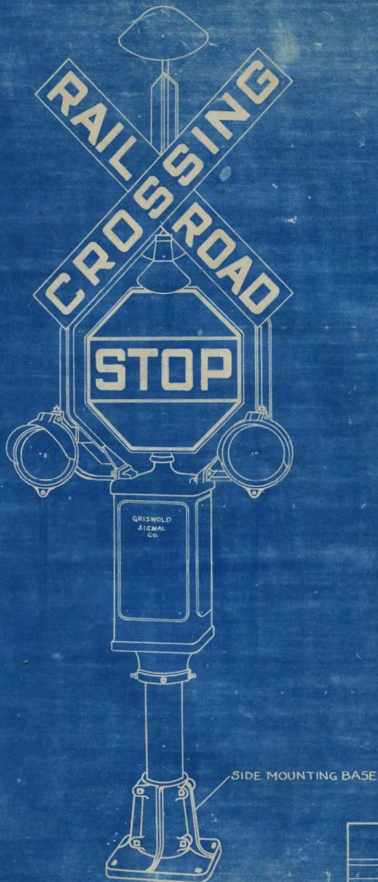
HIGHWAY CROSSING SIGNAL WITH FOUR ADJUSTABLE FLASHING LIGHTS FOR PROTECTING A CROSSING WITH A ROAD APPROACHING AS SHOWN IN THE KEY MAP AT THE RIGHT SPECIFY CENTER OR SIDE MOUNTING BASE
