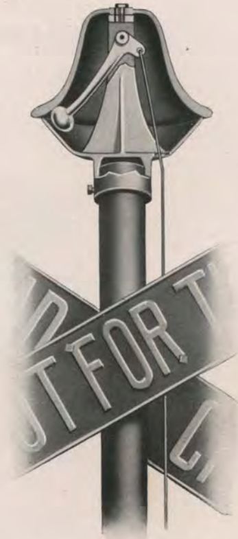
Sectional View of Style C and D Bells
