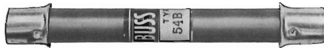
No. 54-A— \frac{25}{64} " Dia., 1\frac{1}{8} " Long; 5 Amperes No. 54-B— \frac{25}{64} " Dia., 3\frac{1}{16} " Long; 2 Amperes
