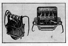
Fig. 115. Shell Type Transformer.
