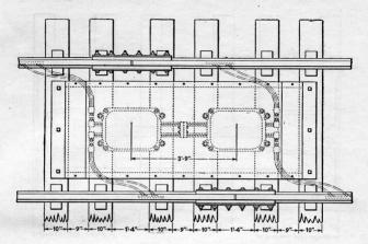
Fig. 100. Double Layout for 1500 Amp. Bond, Fig, 96; the Two Bonds Shown Above are Provided with a Sheet-Iron Cover for Protection Against Dragging Car Rigging.
