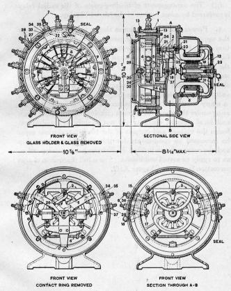
This relay may also be provided with contacts closed only in the de-energized position of the relay; such a contact takes the same space as one complete three-position (pos. and neg.) contact.
