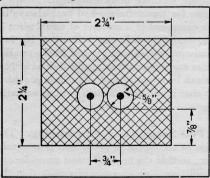
Fig. 186. Conduit for 3300 Volt Single Phase Underground Transmission.
