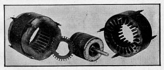
Fig. 145. Elements of the Induction Motor.
