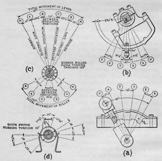
Fig. 210. Diagram Illustrating the Operation of Switch Levers.
