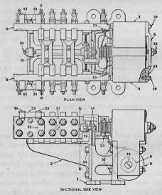
Fig. 218. Polarized Switch Circuit Controllers.
