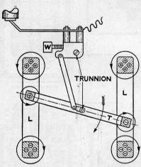
Fig. 48. Magnetic Flux Relationships Ironless Galvanometer Relay.
