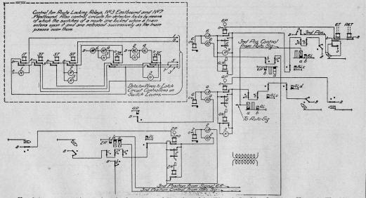
Fig. 228. Control Circuits for Third Position of Signals and for Electric Locking for Plant Shown in Fig. 226.
