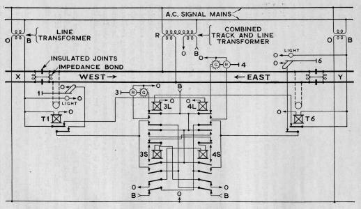
Fig. 200. Circuit Scheme for T. D. B. System.
