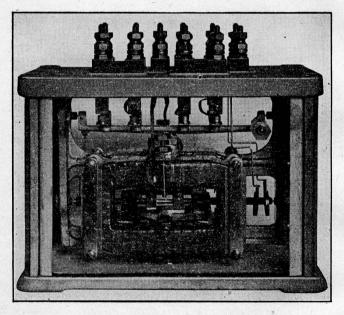
Fig. 45. Ironless Galvanometer Relay.
