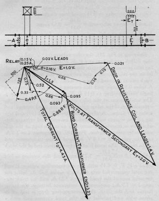
Fig. 241. Vector Diagram For a Track Circuit Equipped With a Polyphase Relay.
