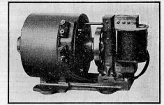
Fig. 150. Induction Signal Motor.
