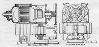
Fig. 152. A. C. Series Commutator Signal Motor.
