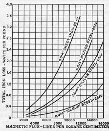
Fig. 112. Iron Loss Curves.
