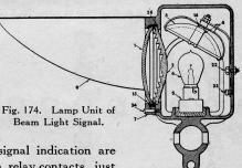
lamps for any signal indication are selected through relay contacts, just as the lamps on an electric sign are
