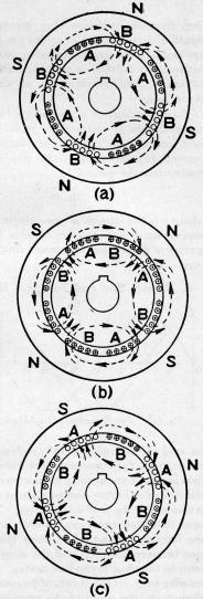
Fig. 147. Production of a Rotating Magnetic Field,
