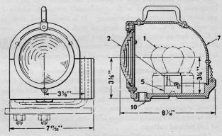
Fig. 156. Semaphore Lamp for Signal Lighting.
