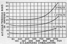
Fig. 89. Unbalancing Curves for a 2000 Amp.
