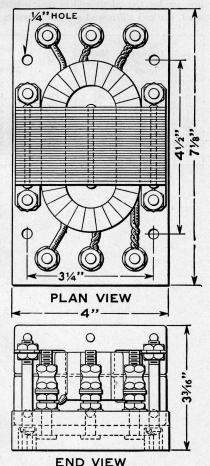
Fig. 137. Track Impedance for Steam or A. C. Electric Roads.
