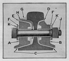
Fig. 234. Model 14 Keystone Insulated Rail Joint.
