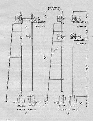
Fig. 167b. One Arm and Two Arm Upper Quadrant Three-Position "T-2"
