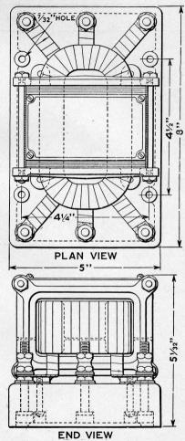
Fig. 139. Track Impedance for D. C. or A. C. Electric Roads. Type B.
