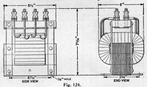
Characteristics. The above transformer is used for feedsteam road track circuits, and is generally provided with a 10volt tap on its primary for feeding signals lamps, relay locals, etc.; the primary cannot be wound for more than 220 volts.
