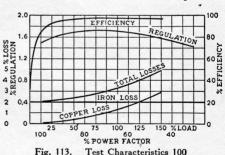
Fig. 113. Test Characteristics 100 K. V. A. Transformer.
