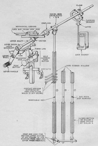
Fig. 213. Perspective Diagram of Signal Lever Complete.
