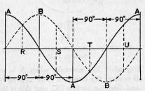
Fig. 66. Quadrature Currents in Polyphase Relay.
