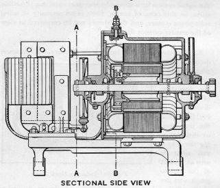
Fig. 151. Cross Section of Induction Signal Motor Shown in Fig. 150.
