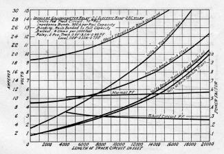
Fig. 53. Power Curves 25 Cycle Ironless Galvanometer Relay on Double Rail Center Fed D. C. Electric Road Track Circuit.
