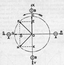
Fig. 67. Illustrating Production of Rotating Magnetic Field.
