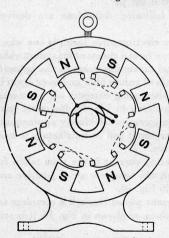
Fig. 20. Armature Winding 8-Pole Alternator
