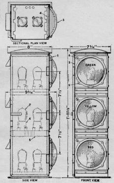
Fig. 178. Three Light Tunnel Signal.
