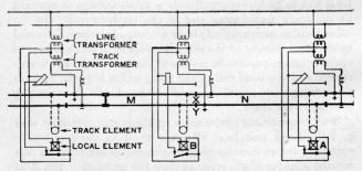
Fig. 33—Two-element, Two-position Relays on an End Fed Track Circuit
