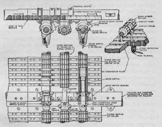
Fig. 214. Section of Combination Plate, Rollers and Contacts.
