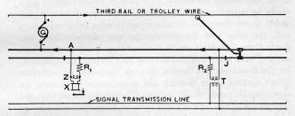
Fig. 86. Single Rail A. C. Track Circuit.
