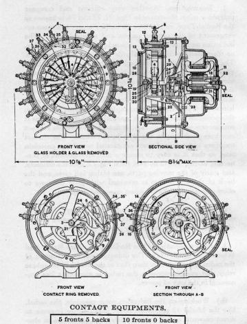
Fig. 73. Two-Position Radial Polyphase Relay.
