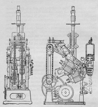
Fig. 159. Style "B" Three-Position A. C. Signal Mechanism.
