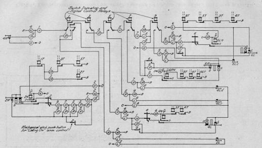
Fig. 227. Signal Control Circuits for Plant Shown in Fig. 226.
