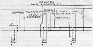
Fig. 31-Element of the End Fed Track Circuit
