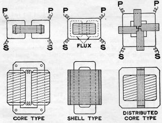
Fig. 114. Types of Transformer Core Construction.
