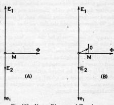
Fig. 168. Vector Diagrams of Transformer Woking on No Load.
