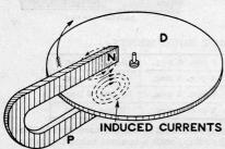
Fig. 65. Metal Disc, Dragged around by Induction.
