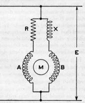
the impressed voltage E, thus counterbalancing, in a way. the inductive effect of the stator winding A; on the other hand, the reactance X is introduced in the right hand circuit to help stator winding B to still further displace the current out of phase with the impressed voltage E. For example, if the total dead resistance in the left hand circuit is 75 ohms. while the inherent reactance of winding A is 25 ohms, then the power factor ( $\cos \theta$ ) of the total left hand circuit is:
