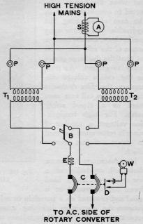
Fig. 195. Circuit Diagram of Interurban Road Switchboard.
