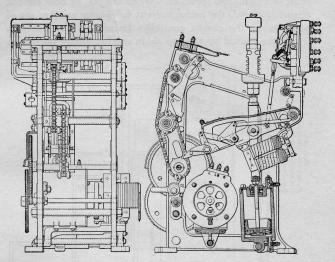
Fig. 162. Mechanism of Style "S" Three-Position Signal.
