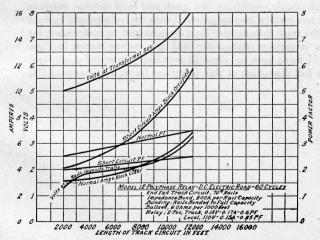
Fig. 71. Power Curves 60 Cycles Model 12 Polyphase Relay on End Fed Double Rail D. C. Electric Road Track Circuit
