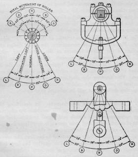
Fig. 211. Diagram Illustrating the Operation of Signal Levers.
