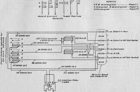
Style ' Three-Position Distant Arm. Circuits for Home and Distant Slot Contact with : Fig. 161.
