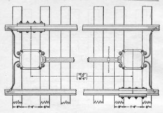
Fig. 102. Double Layout for 500 Amp. Bond Fig. 97. In This Layout the Neutral Connection Between Bonds is Made Long Enough to Eliminate the Necessity of Cutting the Rails to Make the Insulation Joints Come Opposite;
