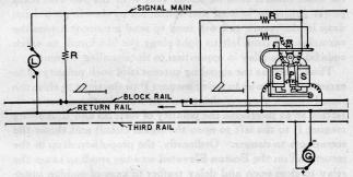
Fig. 2-Boston Elevated Track Circuit
