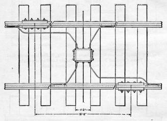
Fig. 106. Layout for Double Bond Shown in Fig. 98. The Rail Cables are Soldered at Their Bond Ends Into Eye Connectors Bolted to the Bond Terminals; the Rail Ends of the Cables are Soldered to U-shaped Connector,
