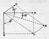
Fig. 25. Determination of Resultant Voltage
