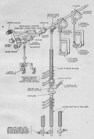
Fig. 212 Perspective Diagram of Switch Lever Complete.
