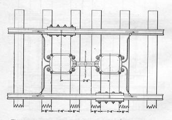
Fig. 103. Double Layout for 500 Amp. Bond Fig. 97. In This Layout the Rails are Cut to Permit the Bonds Being Placed Close Together.
