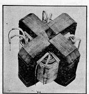
Fig. 116. Distributed Core Type Transformer.
