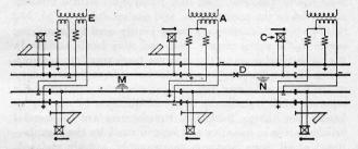
Fig. 35—Multiple Feeding of Parallel Track Circuits
