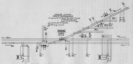
Fig. 226. Complete Layout fo Small Type "F" Interlocking Plant.
