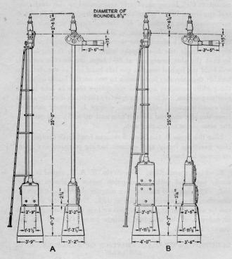
Fig. 163b. One Arm Style "S" Three-Position Upper Quadrant Ground Post Signals. The Signal at the Right is Provided With a Double Case, the Lower Half of Which May be Used for Housing Track Transformers, Impedances or Extra Relays.
