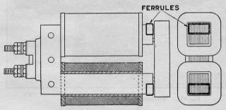
Fig. 153. Tractive Type Slot Magnet.
