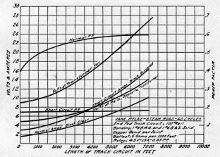
Fig. 42. Power Curves for 60 Cycle Single Element Vane Relay on End Fed Steam Road Track Circuits of Various Lengths.
