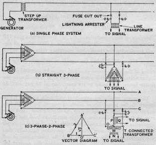
Fig. 182. Diagrams of Three Principal Transmission Systems Used in Signal Work.
