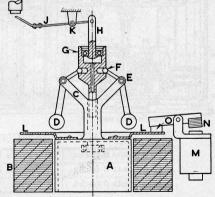
Fig. 78. Operating Mechanism Centrifugal Frequency Relay.
