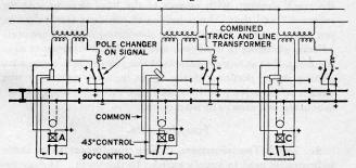
Fig. 34—Polarized Wireless Track Circuit with Three-position Relays
