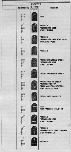
Fig. 176. Beam Light Signal Aspects and Their Meaning.
