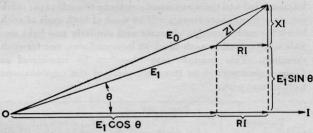
Fig. 181. Initial Voltage Impressed on Transmission Line Divided Into Its Components.
