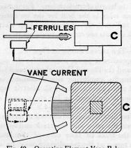
Fig. 40. Operating Element Vane Relay.
