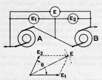
Fig. 24. Vectorial Addition of Voltages
