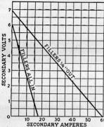
Fig. 121. Characteristics of the Adjustable Filler Transformer.
