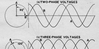
Fig. 183. Wave Traces of Two-Phase and Three-Phase Voltages.
