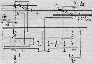
Fig. 225. Check Locking Between Towers.
