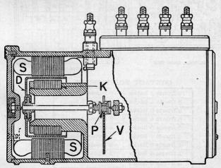
Fig. 62. Operating Mechanism Model 12 Polyphase Relay.
