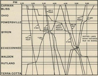
Fig. No. 2—Train Movements by Signal Indication for a 3-Hour Period
