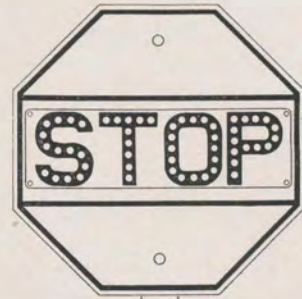
W-103-SIGN 24" Dia. x 1/8" Plate. Letters 1 1/8" Thick
