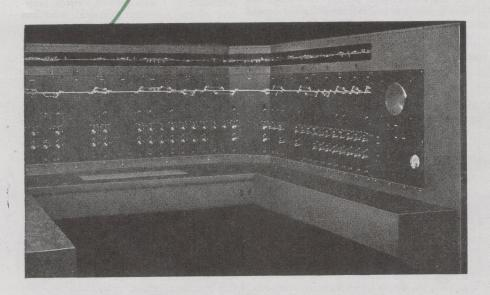
The panel of this G-R-S CTC machine presents a continuous, up-tothe-minute picture of track conditions on the L & N between Welka and Catoma. The operator arranges meets and passes instantly as occasion requires.
