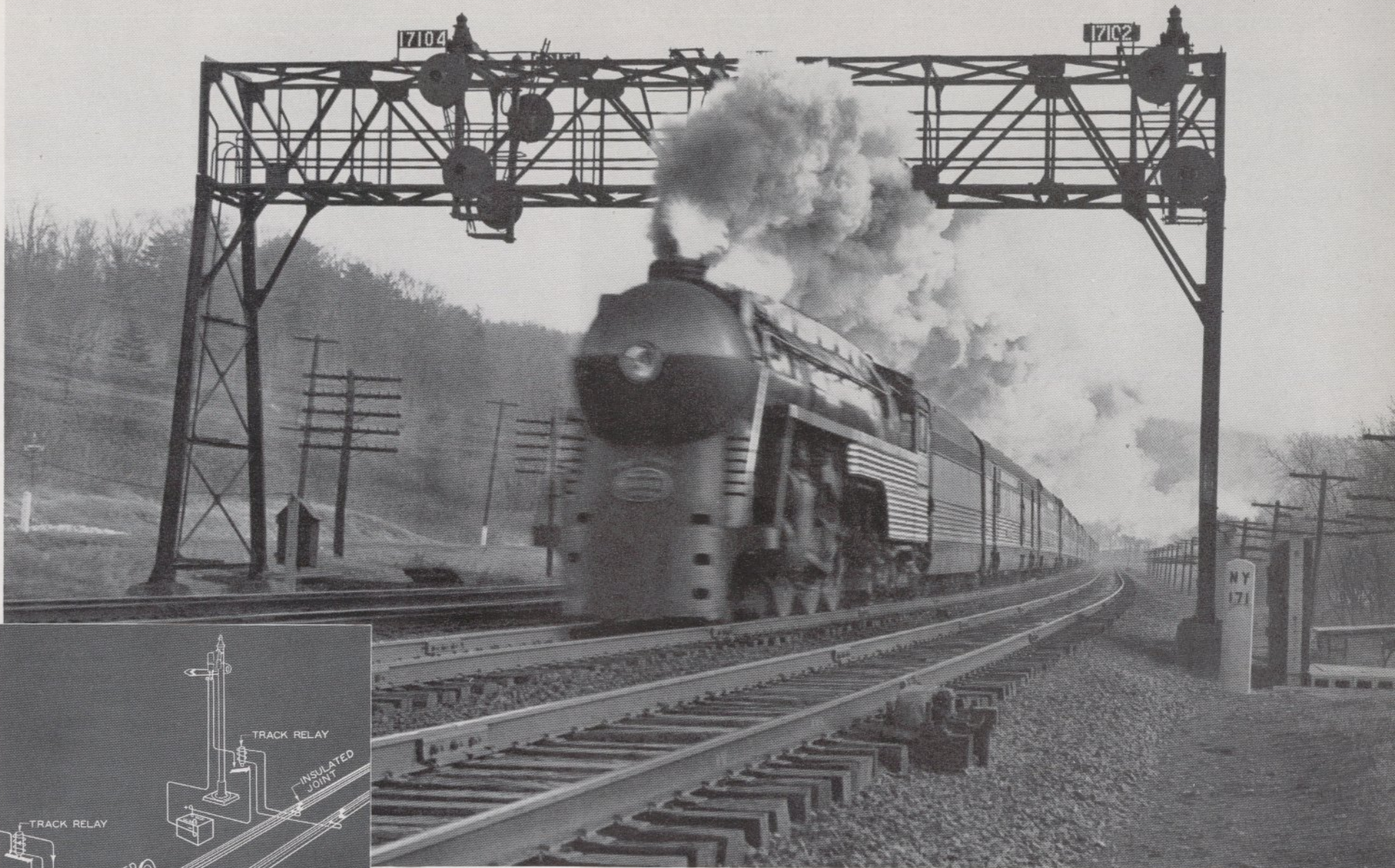
G-R-S automatic block signals and automatic train control permit safe, high-speed operation on this four-track New York Central mainline.
