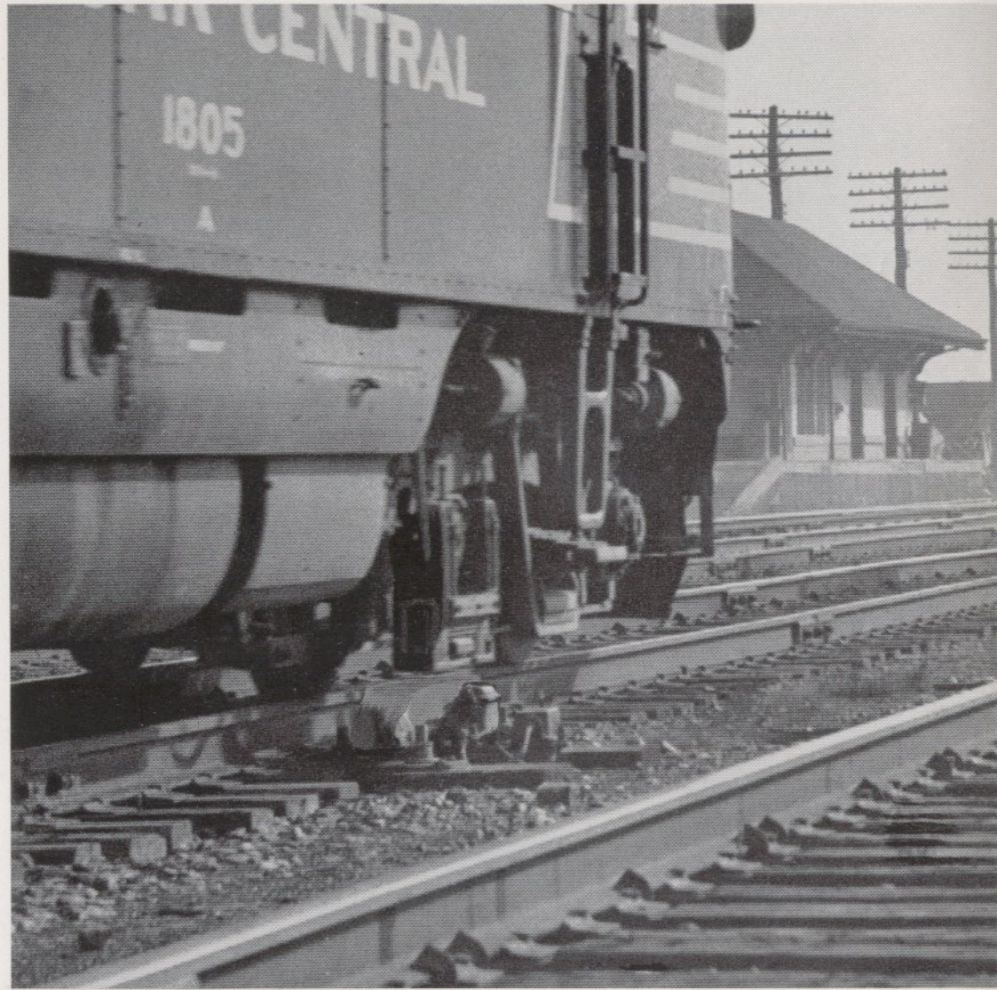
Above: There is no mechanical contact as the receiver passes over the inductor. Invisible magnetic linkages check whether all is clear ahead. Left: Each wayside inductor (shown here in foreground) stands ready to transmit a warning to passing trains if there is danger ahead.
