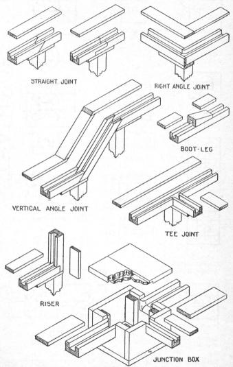
Fig. 271. Trunking and Junction Box Construction
