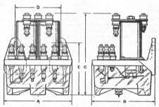
Fig. 229. Model 9, D.C. Relay, Wall Type
