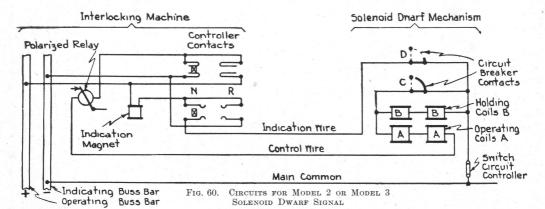
with the operating coils, the flow of current being thereby reduced to the minimum required to retain the arm at proceed. The full movement of the lever to the reverse position is accomplished by means of a local battery indication.
