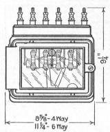
Fig. 235. Model 2 Form A Polyphase Relay
