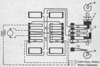
Fig. 147. Pole Changer Wiring, Model 2 Switch Machine
