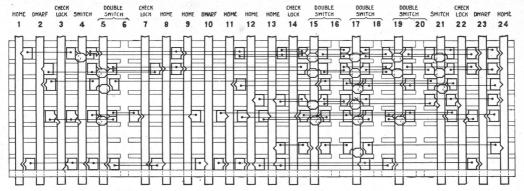
Fig. 34. Dog Chart for Locking in Model 2 Interlocking Machine. Thirty-third Street Station, Hudson Tunnels, H. & M. R. R.
