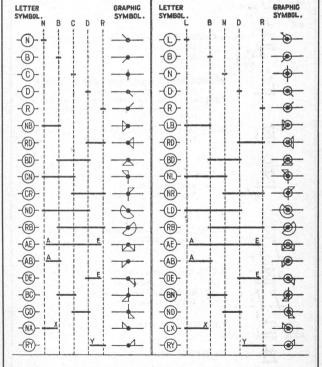
NOTE: HEAVY HORIZONTAL LINES INDICATE PORTION OF CYCLE OF LEVER THROUGH WHICH CIRCUIT IS CLOSED
