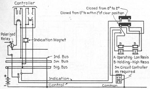
Fig. 225. Typical Circuit for One Arm, Model 2 Solenoid Dwarf Signal
