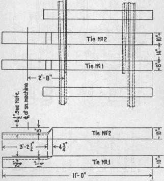
Fig. 149. The Framing for Model 4 Switch Machine
