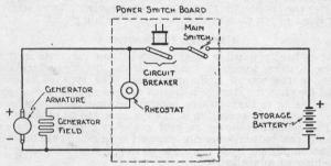
Fig. 110. SIMPLIFIED CHARGING CIRCUIT
