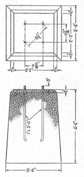
Fig. 216. Ground Signal Mast Foundation R. S. A. drawing 1107, dated 1909. (30.25 cubic feet of concrete.)
