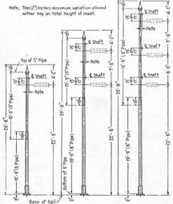
Note; Distance between center of pole and vertical center of shaft to be not less than  $3\frac{5}{6}'''$  nor more than  $4\frac{5}{6}''$
