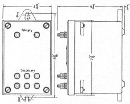
Fig. 249. Type K Secondary Track Transformer
