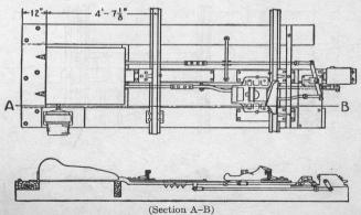
Fig. 167. Hayes Derail Operated by Model 2 Switch Machine
