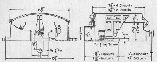
Fig. 185. Dimensions of Model 3 Form D Switch Circuit Controllers
