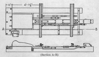
Fig. 169. Wharton or Morden Derail Operated by Model 2 Switch Machine
