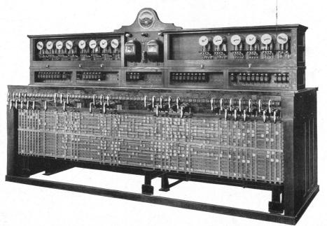
Fig. 32. Unit Lever Type Interlocking Machine in Combination with Operating Switchboard and Indicator Groups. (See Fig. 29.)
