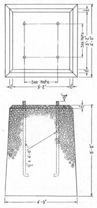
NOTE; 20" for Pipe Bracket Post. 22" for Channel Column Bracket Post.
