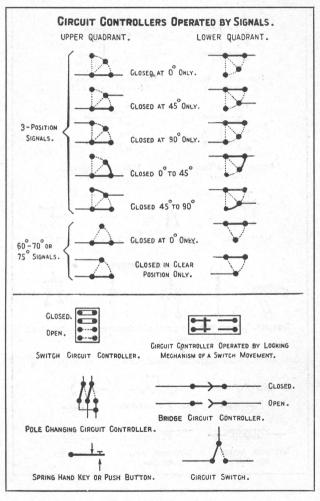
R. S. A. SYMBOLS FOR CIRCUIT CONTROLLERS, RELEASES, ETC.
