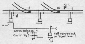
Fig. 100. STICK LOCKING CIRCUIT
