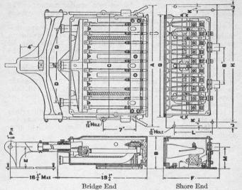
Fig. 195. Bridge Circuit Closer Ten way, controlling ten circuits.
