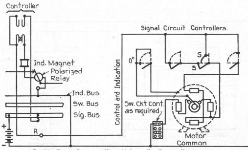
Fig. 220. Typical Circuit for Model 2A Signal, Two Position, Non-Automatic Employing semi-automatic mechanism.
