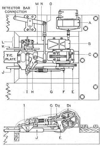
Fig. 43. Model 2 Switch Machine
