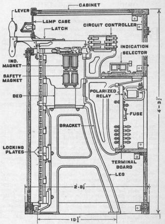
Fig. 136. Model 2 Unit Lever Type Interlocking Machine
