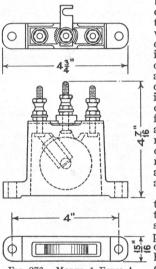
Fig. 276. Model 1 Form A LIGHTNING ARRESTERS
