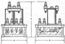
FIG. 228. MODEL 9, D.C. RELAY, SHELF TYPE
