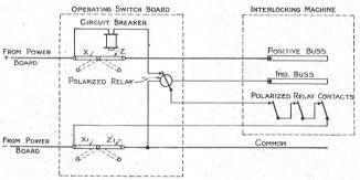
Fig. 26. Simplified Circuits for Operating Switchboard Lettering of the cross protection circuit breaker contacts corresponds with the lettering used in Figs. 64 and 66.
