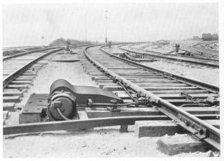
Fig. 40. Model 2 Switch Machine. Buffalo Creek Inter-Locking Plant, L. S. & M. S. R'Y
