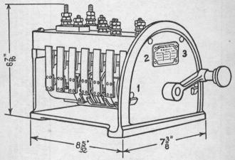
Fig. 108. BATTERY CHARGING SWITCH
