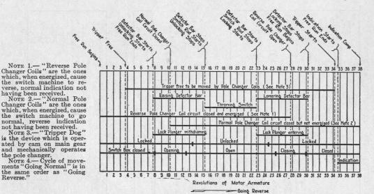
Fig. 155. Cycle of Movements of Model 4 Switch Machine
