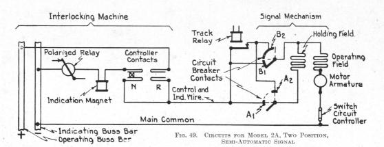
will continue its movement, current being taken through the track relay contact and circuit breaker contact  $B_2$ ; the movement of the mechanism from the zero degree position on, carries the semaphore blade with it to the proceed position. Just before reaching this position circuit breaker contact  $B_2$  opens, and  $A_2$  closes, again cutting the holding field in series with the operating field and armature, thereby retaining the signal mechanism and signal arm in the proceed position.
