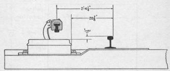
Fig. 157. Diagram Showing Clearance between Top of Model 4 Switch Machine and Contacting Surface of Third Rail. Electric Division, N. Y. C. & H. R. R. R.
