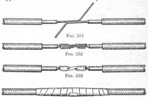
${\rm Fig.~254}$  Splicing Stranded Wire to Stranded Wire
