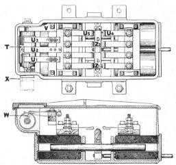
Fig. 42. Pole Changer for Model 2 Switch Machine
