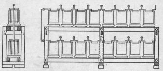
Fig. 105 LEAD Type Storage Battery and Battery Rack
