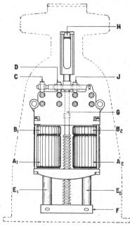
Fig. 63. Model 3 Solenoid Dwarf Signal Operating Mechanism
