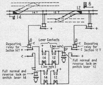
Fig. 98. ROUTE LOCKING CIRCUIT
