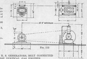
INSTALLATION DATA FOR G. R. S. GENERATORS, BELT CONNECTED TO FAIRBANKS-MORSE VERTICAL GAS ENGINES
