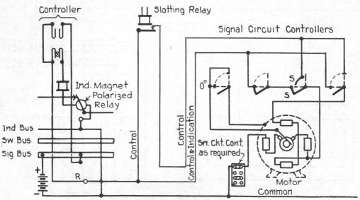
Fig. 222. Typical Circuit for Model 2A Signal, Two Position, Semi-Automatic Controlled through slotting relay in the interlocking station or at point in the field other than at the signal location.
