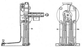
Fig. 55. Dwarf Bearing for Model 2A Signal Mechanism
