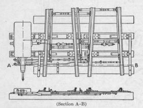
Fig. 172. Double Slip Switch Operated by Model 4 Switch Machine
