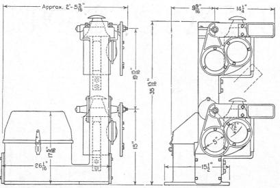
Fig. 206. Dimensions of Two Arm Model 2 Solenoid Dwarf Signal Spectacle R. S. A. drawing 1233, October, 1912.
