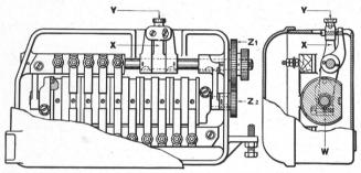
Fig. 47. Switch Circuit Controller for Model 4 Switch Machine
