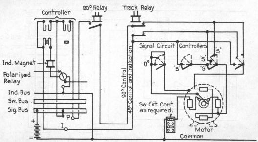
Fig. 223. Typical Circuit for Model 2A Signal, Three Position, Semi-Automatic Controlled through track (slotting) relay located at the signal.
