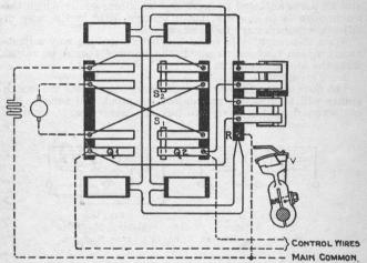
Fig. 153. Pole Changer Wiring, Model 4 Switch Machine
