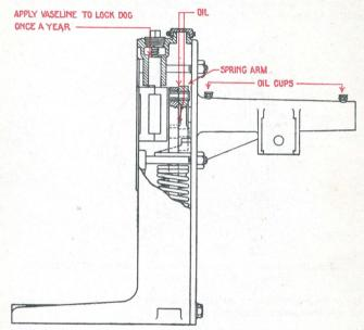
Fig. 198. Oiling Diagram for Model 2A Dwarf Bearing
