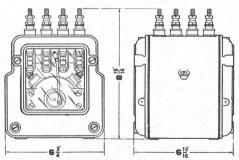
Fig. 231. THREE Position D. C. Motor Relay
