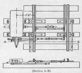
Fig. 162. Single Switch Operated by Model 4 Switch Machine
