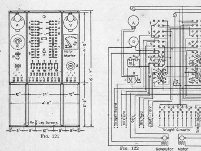
Power Switchboard for One D.C.-D.C. Motor Generator Set, One 110 Volt Battery (No. 1), Two 10 Volt Batteries (Nos. 2 and 3), One Automatic Signal Battery (No. 4) and Two Sets of Track Batteries (Nos. 5 and 6)
