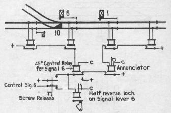
Fig. 99. Approach Locking Circuit
