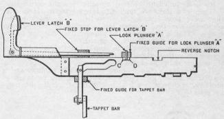
Fig. 139. Notching of Lever for Lever Lock. Normal Position
