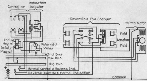
Typical Circuits for Model 4 Switch Machine
