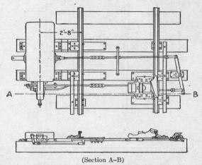
Fig. 166. Hayes Derail Operated by Model 4 Switch Machine
