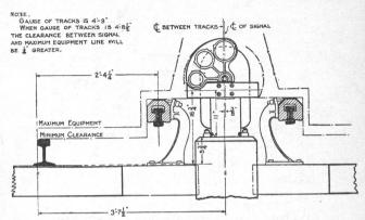
Fig. 202. Diagram Showing Clearance between Model 2A Dwarf Signal and Third Rail. Electric Division, N. Y. C. & H. R. R. R.
