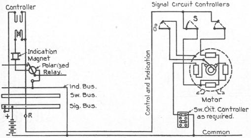
Fig. 219. Typical Circuit for Model 2A Signal, Two Position, Non-Automatic
