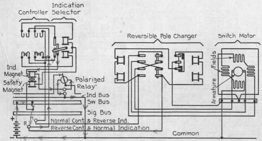
Fig. 178. Typical Circuits for Model 2 Switch Machine
