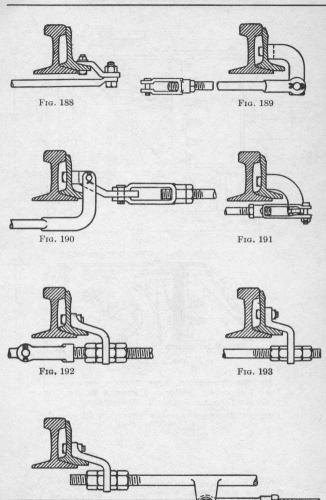
Connections from Switch Point to Switch Circuit Controller
