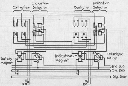
Fig. 180. Wiring Diagram for Cross Connecting the Indication Circuits of Double Switch Levers
