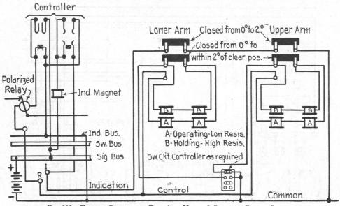
Fig. 226. Typical Circuit for Two Arm, Model 2 Solenoid Dwarf Signal
