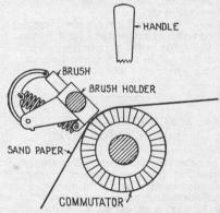
Fig. 111. Method of Fitting Brushes to Commutator
