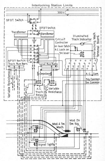
Fig. 90. Section of Interlocking Plant Showing use of central energy scheme for track circuit control.
