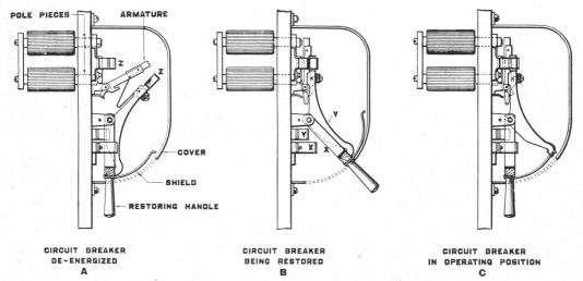
Fig. 66. Sectional View of Cross Protection Circuit Breaker Parts similarly lettered make contact with each other.
