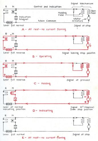
Fig. 8. Simplified Circuits for Model 2A, Non-Automatic, Two Position Signal
