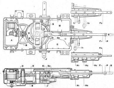
Fig. 44. Model 4 Switch Machine Showing single and double locking cages.
