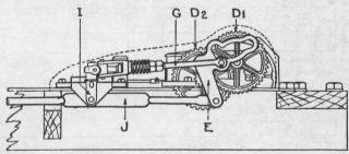
Fig. 143. Model 2 Switch Machine
