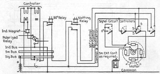
Fig. 224. Typical Circuit for Model 2A Signal, Three Position, Semi-Automatic Controlled through slotting relay in the interlocking station or at a point in the field other than at the signal location.
