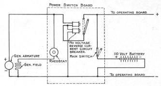
Fig. 22. Simplified Circuits for Power Switchboard
