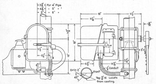
Fig. 199. Dimensions of Model 2A Semi-Automatic Signal Wires carried from mast to signal mechanism in flexible conduit (see Fig. 203).
