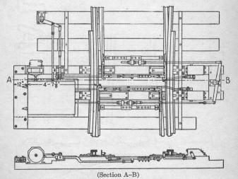
Fig. 175. Movable Point Frog Operated by Model 2 Switch Machine
