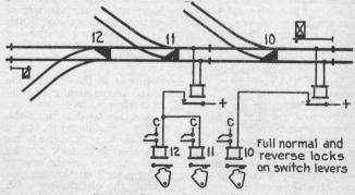
Fig. 97. Section Locking Circuit
