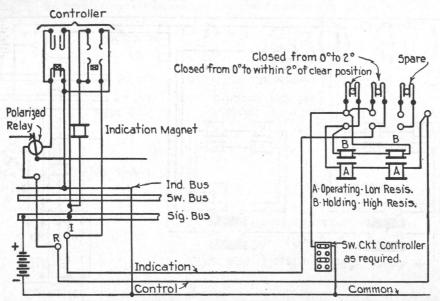
Fig. 227. Typical Circuit for Model 3 Solenoid Dwarf Signal
