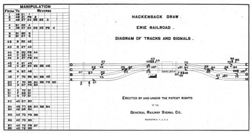
FIG. 79. TRACK DIAGRAM AND MANIPULATION CHART. HACKENSACK DRAW BRIDGE, ERIE R. R.
