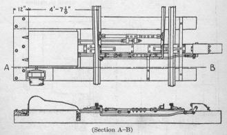
Fig. 163. Single Switch Operated by Model 2 Switch Machine
