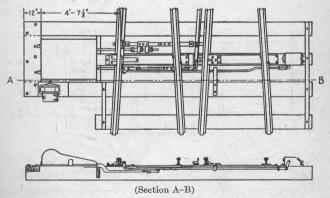
Fig. 171. Single Slip Switch Operated by Model 2 Switch Machine
