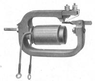
Fig. 67. Polarized Relay
