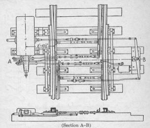
Fig. 174. Movable Point Frog Operated by Model 4 Switch Machine
