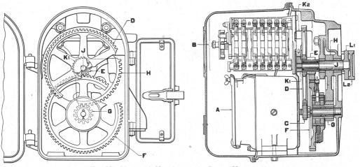
Fig. 52. Model 2A Non-Automatic Signal Mechanism
