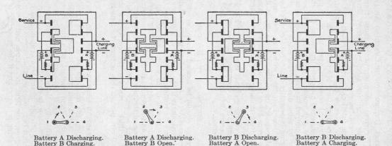
FIG. 109. DIAGRAM OF CONNECTIONS MADE AT THE DIFFERENT OPERATING POSITIONS OF THE BATTERY CHARGING SWITCH
