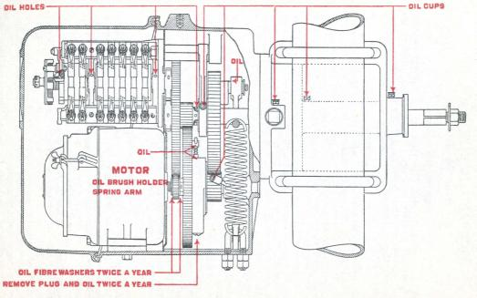
Fig. 196. Oiling Diagram for Model 2A Semi-Automatic Signal Mechanism and Clamp Bearing
