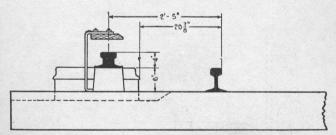
Fig. 158. Diagram Showing Clearance between Top of Model 4 Switch Machine and Contacting Surface of Third Rail, Long Island R. R.
