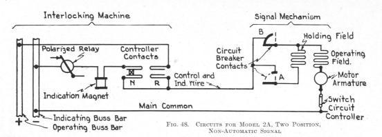
signal arm in the desired position so long as the circuit is intact. Since the holding field windings have a high resistance the current used to hold the signal in the proceed position is reduced to a minimum.
