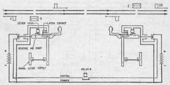
Fig. 103. Check Locking Circuit
