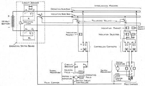
Fig. 64. Circuits for Operating Switchboard, Interlocking Machine and Switch and Signal Functions
