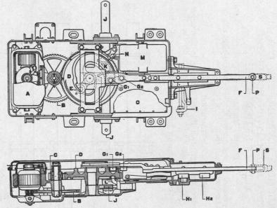
Fig. 150. Model 4 Switch Machine
