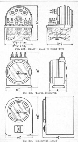
Model 2 Form B, Model 3 Form B, or Model Z Form B, A. C.
