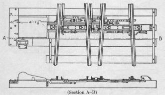
Fig. 173. Double SLIP Switch Operated by Model 2 Switch Machine
