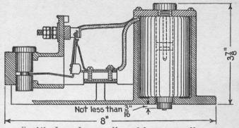
Fig. 141. Lever Lock for Model 2 Interlocking Machine
