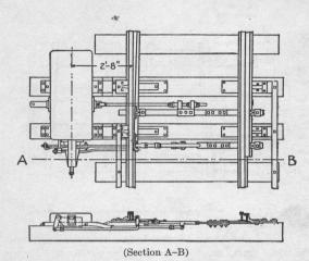
Fig. 168. Wharton or Morden Derail Operated by Model 4 Switch Machine
