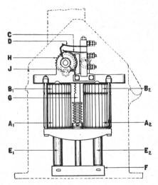
Fig. 61. Model 2 Solenoid Dwarf Signal Operating Mechanism
