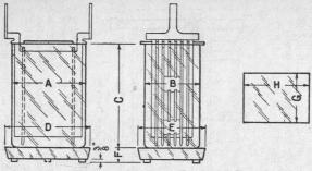
Fig. 106. Battery Jar, Sand Tray and Cell Cover DIMENSIONS AND WEIGHTS OF LEAD TYPE STORAGE BATTERY CELLS
