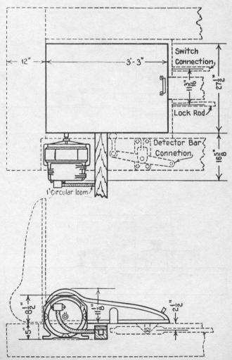
Fig. 159. DIMENSIONS OF MODEL 2 SWITCH MACHINE
