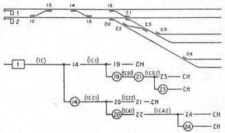
Fig. 275. Signal Selecting Circuit
