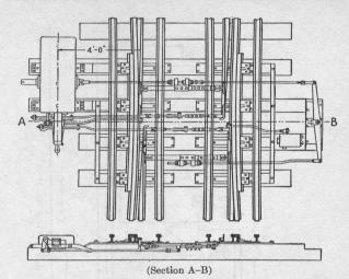
Fig. 176. Movable Point Frog (with Double Slip Switch)
