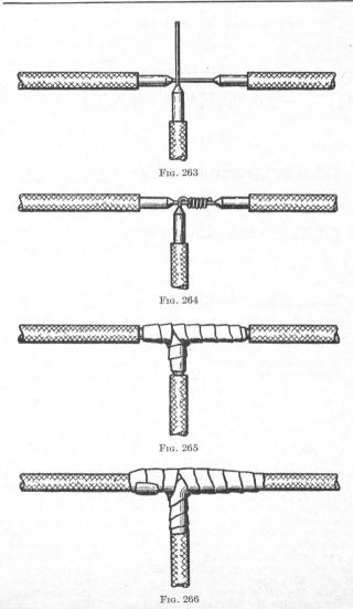
MAKING T JOINTS IN SOLID WIRE
