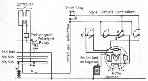
Fig. 221. Typical Circuit for Model 2A Signal, Two Position, Semi-Automatic Controlled through track (slotting) relay located at the signal.
