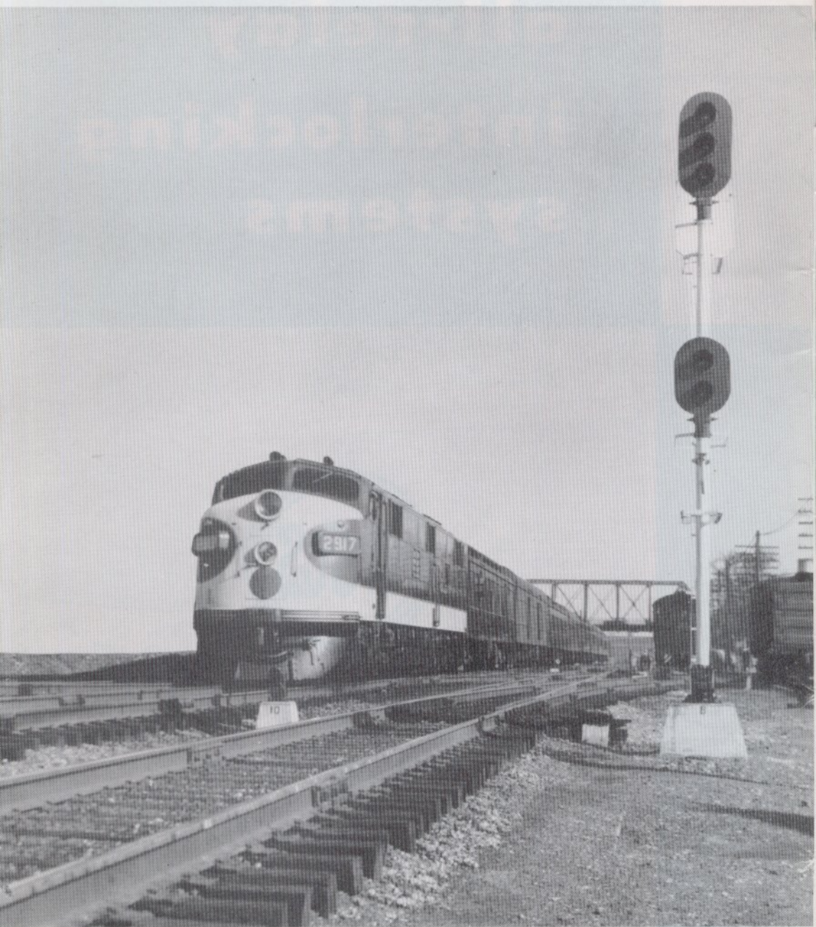
NX interlocking facilitates heavy traffic involving as many as 500 line-ups a day at Howell, Georgia, on the Nashville, Chattanooga and St. Louis Railway.
