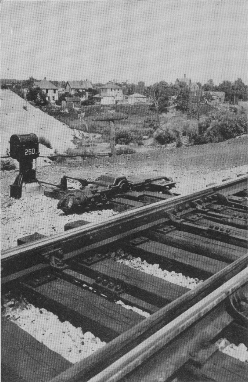
Figure 8. This Model 9A switch lock locks the selector lever on a G-R-S Model 5D dual-control electric switch machine.
