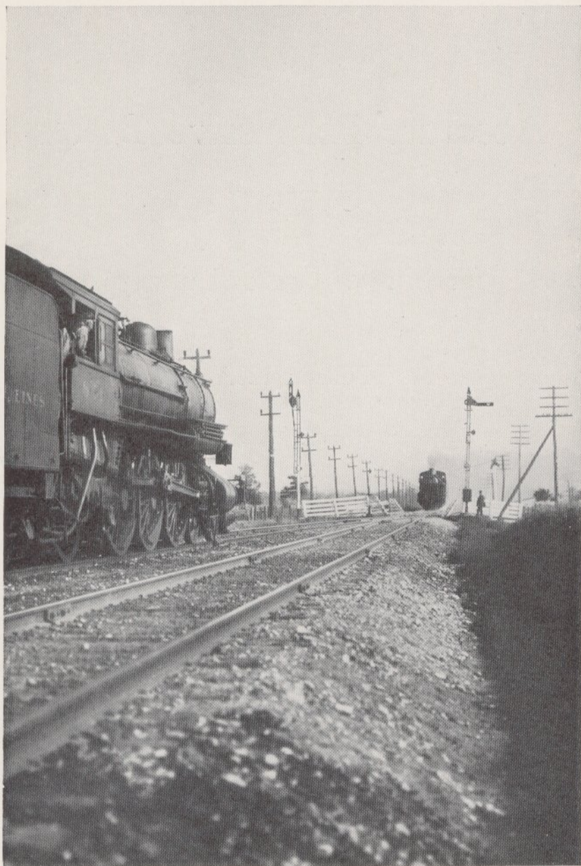
A-P-B System on the Toronto, Hamilton & Buffalo Railway. Trains 73 and 78 meeting at Grassies, Ont. This road was the first to install the A-P-B System
