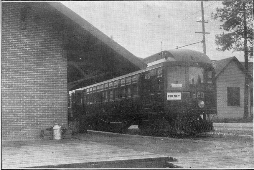
Fig. 11. Car Showing Automatic Stop Tube.
