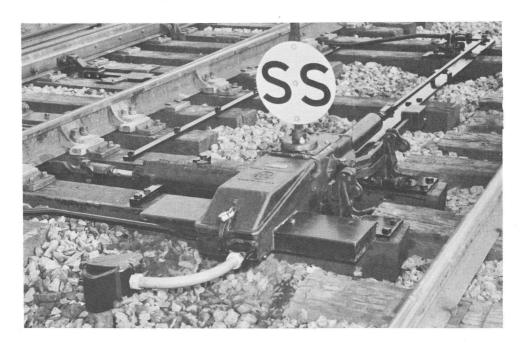
Typical spring switch installation. Low target staff with "SS" marker is optional equipment.
