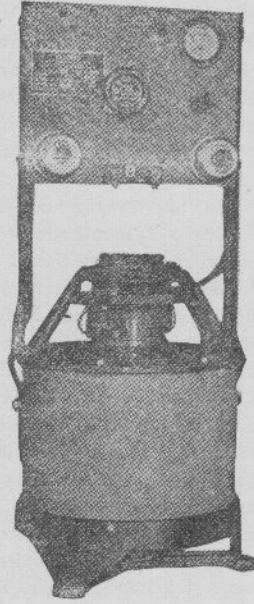
Fig. 2. Automatic Motor-Generator Set.
